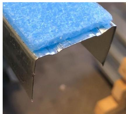
The profiles are available with different types of surface treatment. This profile for use in internal walls and ceilings has a surface layer of 100 g per square meter.
