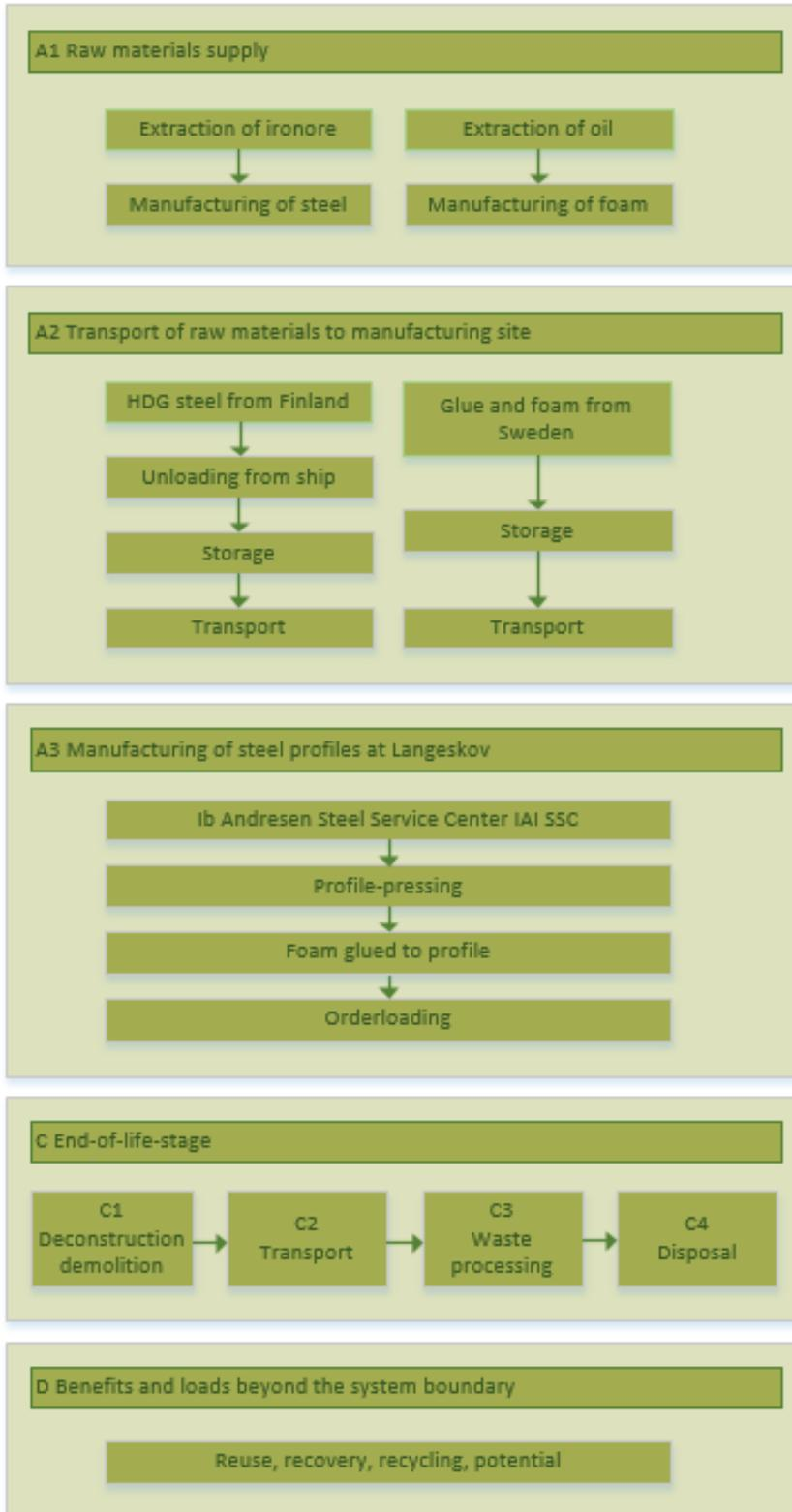
The profiles are manufactured from hot dip galvanized carbon steel delivered from steelworks as coils by boat to the IAI's port in Nyborg. In IAI site Langeskov, the coil is divided in narrow bands whose width fit the specific profiles, and the profiles are manufactured through roll forming technique. Sheets of insulation foam is glued to the profiles.
