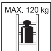
Max. load for the ladder is 120 kg.
