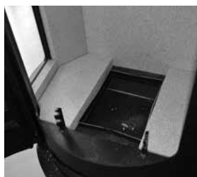
Fit base right and left bricks, place grate support in central position.
