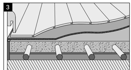
Laminate Flooring on Duo-Protect / Hot watertype subfloor heating
