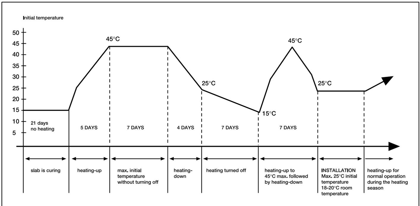
Keep in mind that the optimum surface temperature of your laminate flooring should not exceed 25°C (maximum 28°C).
