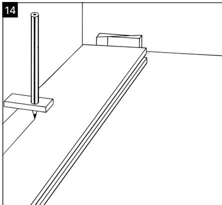
**Fig. 15:** How to shorten a door frame: place a piece of residual board on top of the underlay against the frame (décor side down) and saw the frame off along the board.
