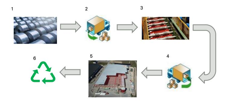
The steel coils (1) are produced at the steel manufacturer and transported to Lindab Profile in Denmark by truck (2). The profile is formed in a rolling machine (3). The production is a pull system (produced to customer order) to reduce waste of the life cycle. Transport to customer is by truck (4) to the building site where the customer assemble the product (5). The usage phase is excluded in this EPD, and that is why the next step is demolition and recycling (6).
