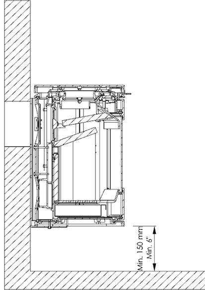
**Note: The supplied wall-mounting fixture is not designed to carry the weight of a heavy chimney as well.**
