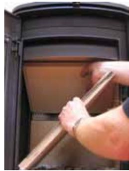
3. Tilt one of the side brick panels and remove it.
