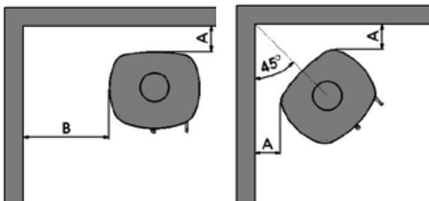
We recommend that the stove be installed at least 10 - 15 cm from masonry, in order to allow heat to circulate and to facilitate the cleaning of the inside and outside of the stove. A layer of wallpaper on a brick wall is normally viewed as non-flammable material.
