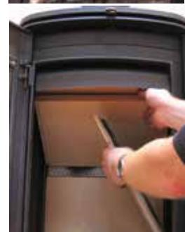
4. Once the side brick panels have been removed, lower the bottom baffle and lift it out.
