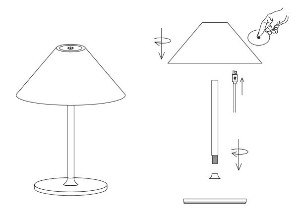
When pressing the on/off indicator, the light will dim up/ down.
