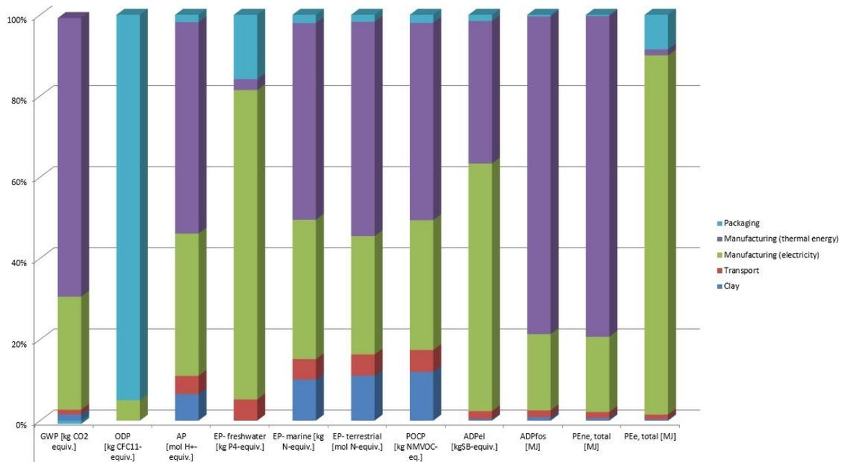
The evaluation of the Life Cycle Assessment results of the roofing tiles shows that the environmental impacts in all environmental categories are dominated by energy consumption during the manufacturing process
