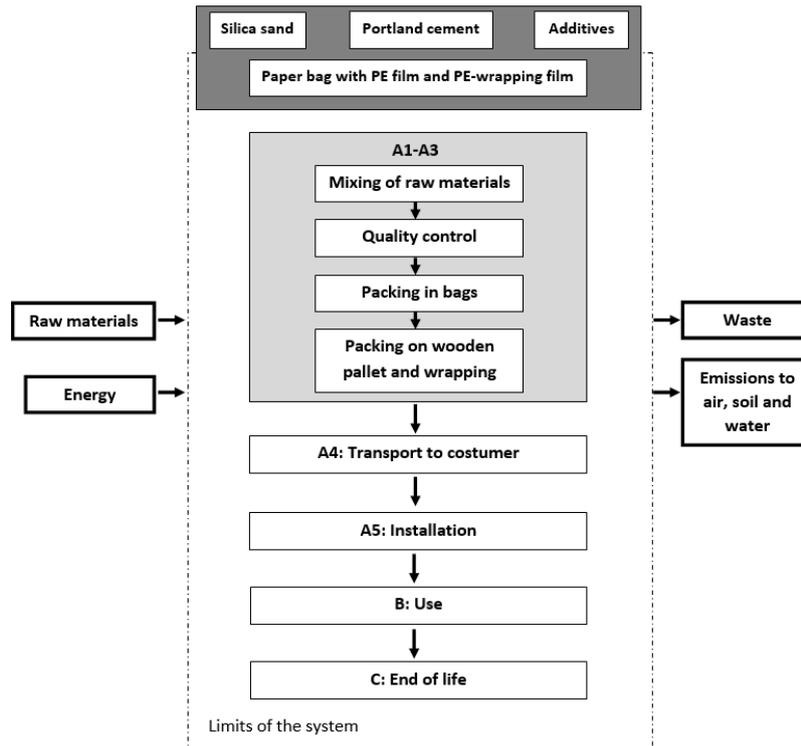
Figure 2: Limits of the system in this study.
