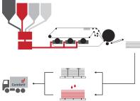
A very thin slurry of water, binder and fibres is mixed and introduced into each of the vats of the Hatschek machine. The rotating sieve cylinder in the vats collects a thin layer of solid material that is further dewatered as it is transferred to a felt and further on to an accumulating format roller. At the required thickness, the accumulated layers are automatically
