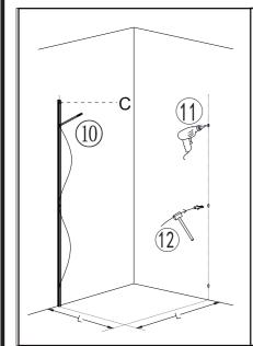
Mark the drill holes on the wall though the holes on the wall profiles
