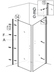
After installed wall profiles put glass door inside wall profiles screw glass door and wall profiles cover the screw cap
