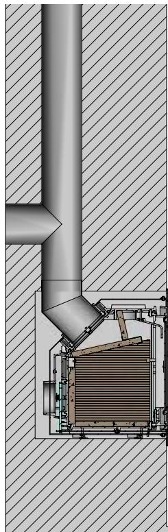
Morsø 5600 connected to existing masonry chimney
