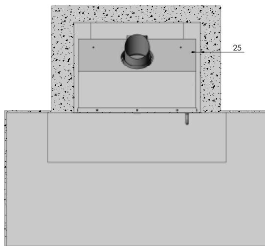
If the insert is installed in a flammable environment, a fireplace structure must be built where the insert may be mounted. The fireplace structure will protect the surroundings against the heat effects of the insert through shielding and ventilation. There are numerous ways to build a fireplace structure.
