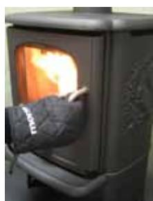
8. Once the new fuel has taken, adjust the secondary air amount to the desired setting; optimal combustion will continue until glowing charcoals are produced. Under normal chimney draft conditions, expect to refuel your stove every 70 - 80 minutes.
