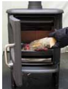
7. When the primary air supply is opened all the way and the door is closed, the new fuel will ignite in a few minutes.
