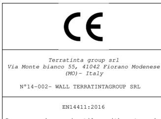
Dry pressed ceramic tile, with water absorbtion Eb > 10% for internal walls.
