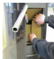
5. Lift the bottom baffle plate free of the tertiary combustion air box and remove it.
