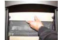
8. Re-installing vermiculite parts: as removal but in reverse order.
